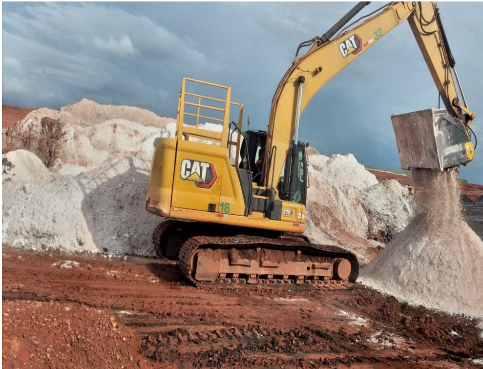
Figure 5. Crushing all the hydrate to homogenize the granulometry.
